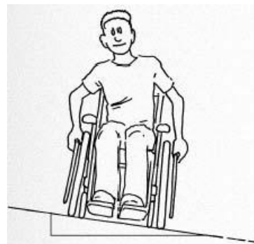
Wheelchair Users Find Severe Cross Slopes Difficult to Navigate
