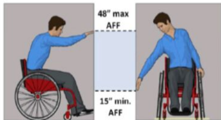
Unobstructed forward and side reaches
