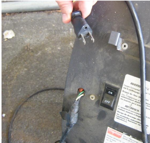
Picture 1: The Plug Is Missing A Ground Prong & The Cord Has Been Pulled From The Device
