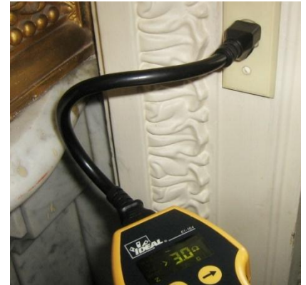
Picture 2: Displays Receptacle With High Impedance
